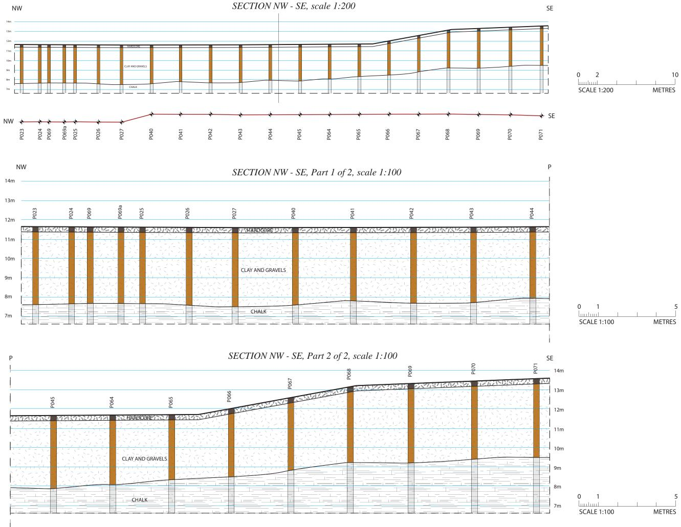
Figure 3: Cross - section NW - SE of the site.
